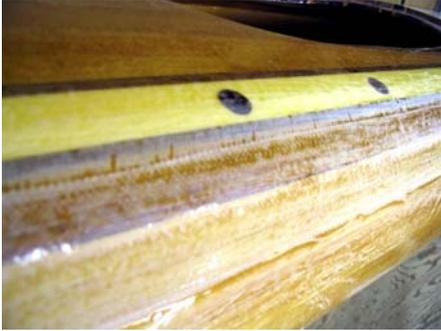
After both sides have cured, scrape and sand down rough edges (**Photo #10**) and apply two more coats with a small brush and smooth with a section of roller. Remember to tip off to prevent bubbles forming. (**Photo #11**)
