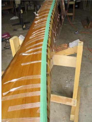
Attaching the deck to the hull can be difficult and frustrating work, especially if your hull or deck has become mis-shaped over time. (See **Fiberglassing** for hints on how to prevent this) You will probably benefit from a second pair of hands for this job.
