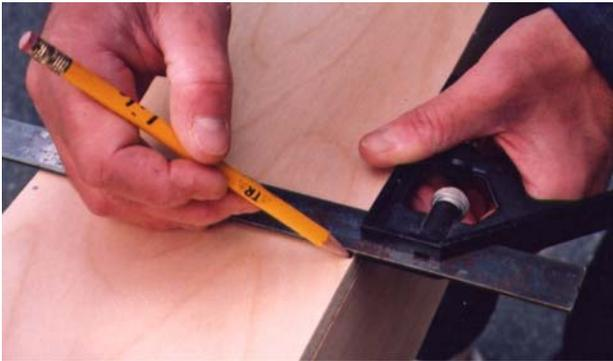
Measure out the box beam in increments as outlined in your plans and mark with a T-square across the beam. **(Photo #2)**
