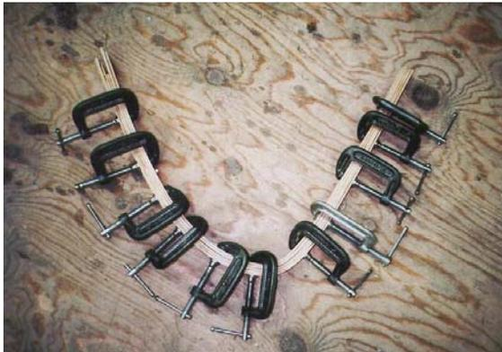
Steam the four or five pieces in a steam tube for at least 20 minutes and then quickly remove and bend around the two forms and clamp overnight.
