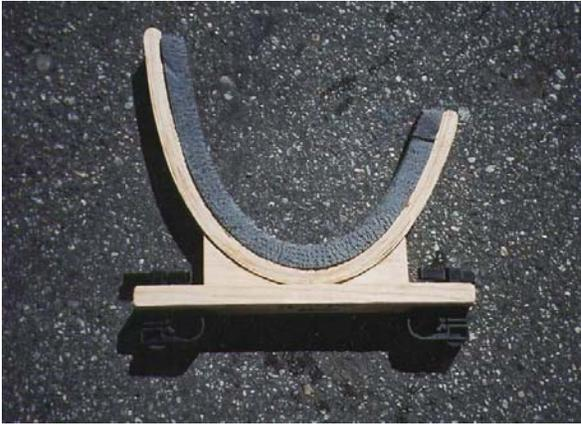
Once you brackets are finished, seal all the wood with several coats of epoxy to protect them from water damage.
