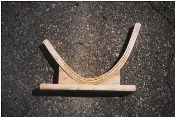
After the two cradles are glued up, clean up all the edges and plane smooth. From another piece of hardwood (1 in. thick by 2 in wide), cut a piece about two feet long. This piece will form the bottom edge that will sit on your roof rack bar. Cut four support pieces that will span the gap on the sides **Photo #3**. Glue the four pieces together with epoxy and also set a few good wood screws through the pieces and up through the bottom for extra strength.
