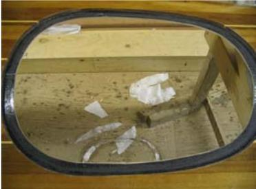
Apply your gasket seal to the hatch lip, to the hatch lid or both.
