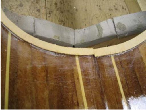
Now cut out full rings per hatch with extra material that will extend into the opening by at least one and a half inches and extend under the deck by a little less than the other rings so there is a small step from layer one to layer two.
