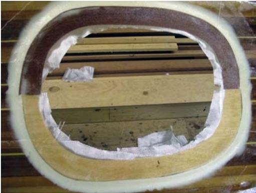
After it has fully hardened, scrape and sand down the rough edges and apply more epoxy to smooth it out. Let harden.
