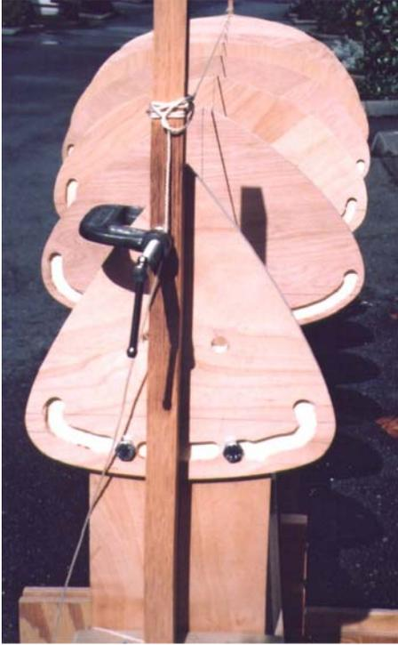
You can also use string lines to check alignment. Clamp a straight piece of wood to the last two forms and align with the vertical centerline. **(Photo #4 & #5)**
